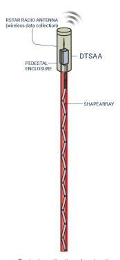
Typical application showing the DTSAA collecting data wirelessly from a ShapeArray instrument in an RSTAR or Stand-Alone Data Logging.
